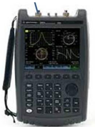
Agilent FieldFox N9918A 5 kHz – 26.5 GHz
