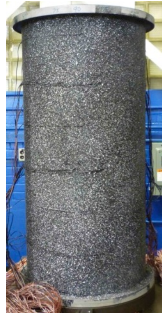
Crown / keel radial deflections measured with VIC3D
