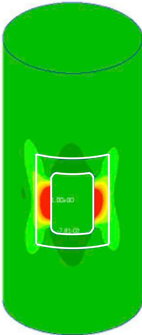
Local buckling - mode 1 (both Shells)
