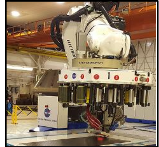
Figure 1. NASA LaRC AFP equipment during fabrication of ACP defect panels
