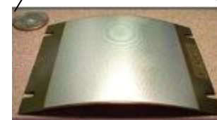
Thin Layer Composite Unimorph Ferroelectric Driver and Sensor (THUNDER)
