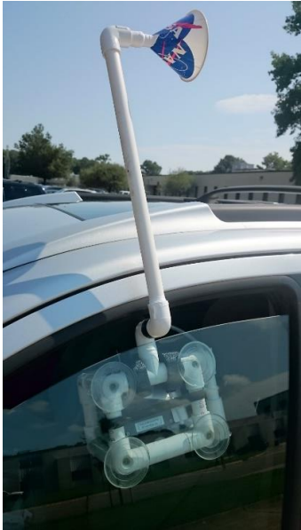
Car in-situ ozone sensor Configuration
