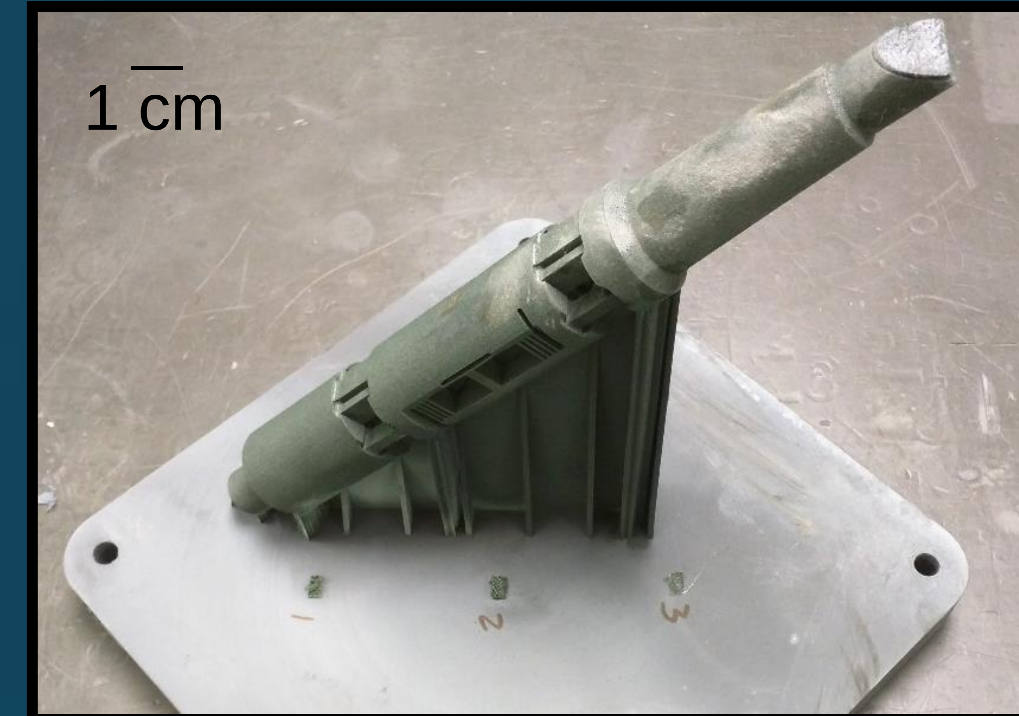
AM force balance (left) as designed (right) printed.
