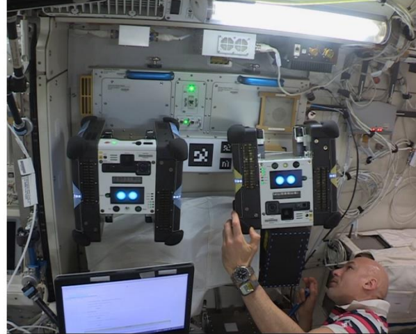
Free-Flyers “Bumble” and “Honey” attached to the Dock inside the Japanese Experiment Module (JEM) Kibo
