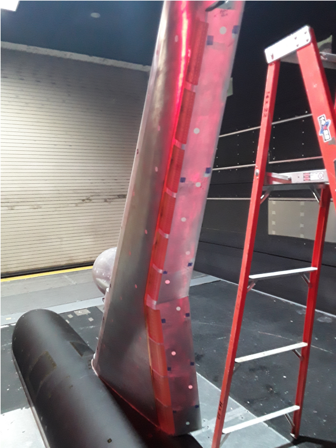
Fig. 18 Wind-tunnel model with Kulites® (covered by blue rectangles) installed on flaps.
