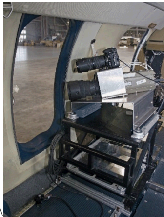
Figure 2: Camera mount used for flight testing.
