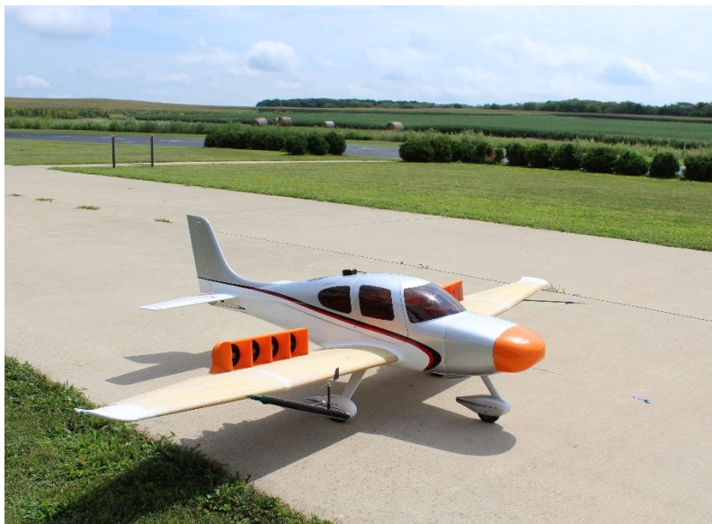
Fig. 17. ADEPT-FC aircraft: 21 percent-scale Cirrus SR22T distributed electric propulsion testbed for propulsion-based control, used with permission by University of Illinois at Urbana-Champaign, Urbana, Illinois.
