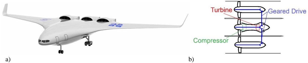
Fig. 4. SAX-40 concept aircraft, a) isometric view from Liu [9], reprinted by permission of the Cambridge University Press; b) sketch of geared drive system for ducted fans.
