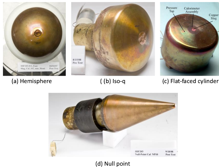
Figure 3.29. Standard calorimeters, (a) Hemi-sphere, (b) Iso-q, (c) Flat-face cylinders and (d) Null point calorimeters. A small copper slug (or Gardon gauge) is located at the center of each of the first three oxygen free copper calorimeters. The null point calorimeter has a very small (and quick
