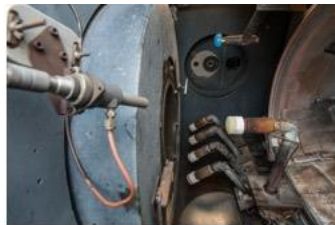
Typical test setup in the AHF with 5 sting arms (5 test articles)
