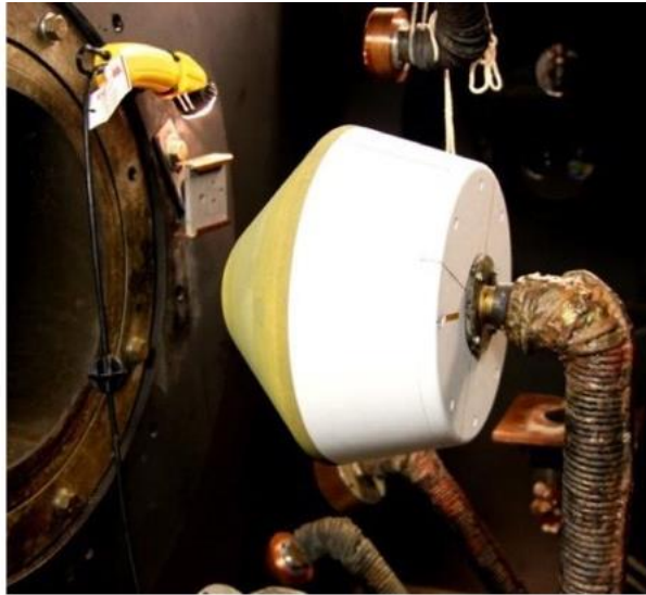
Figure 3.40. Sting mounted test article in the arc jet prior to testing [90].
