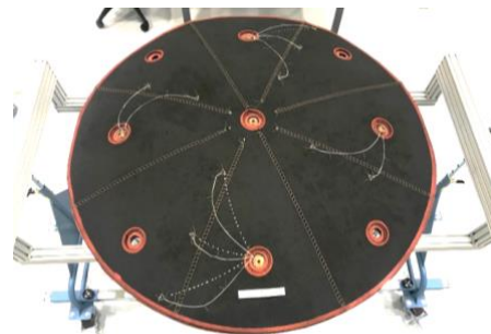
Fig 1. Thermocouples and Heat Flux Gages Integrated with LOFTID Nose Insulation.
