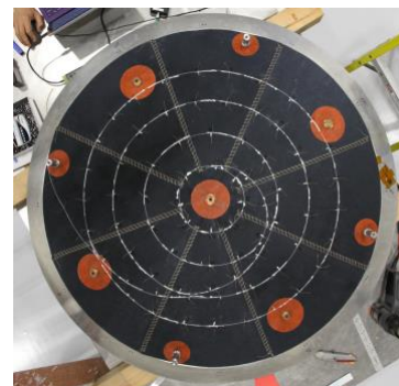
Fig 2. FOSS Installed between Insulation Layers on LOFTID Nose.
