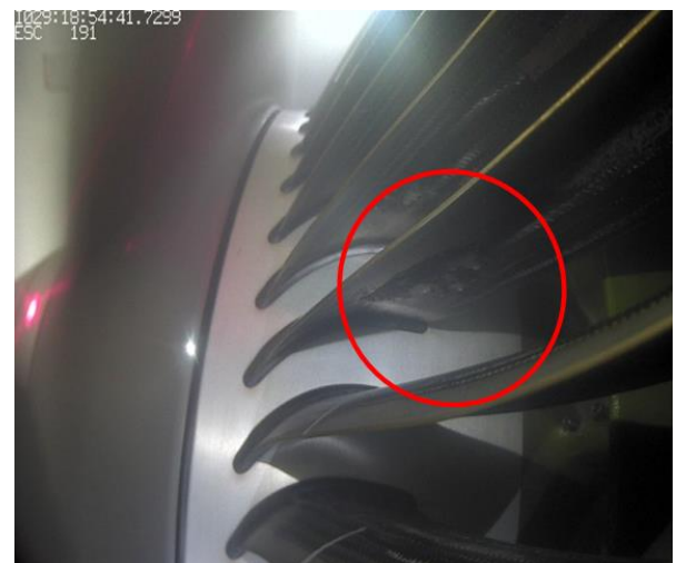
c.) Reading 191, MVD = d_{v,0.50} = 114 \mu\text{m}
