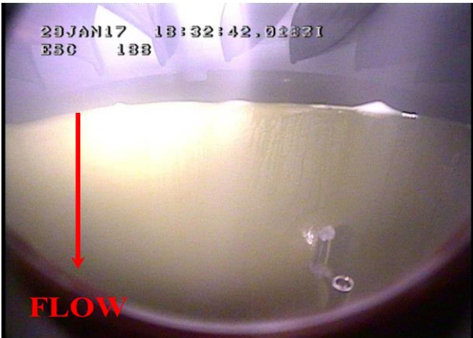
a.) Reading 188, MVD = d_{v,0.50} = 15 \mu\text{m}
