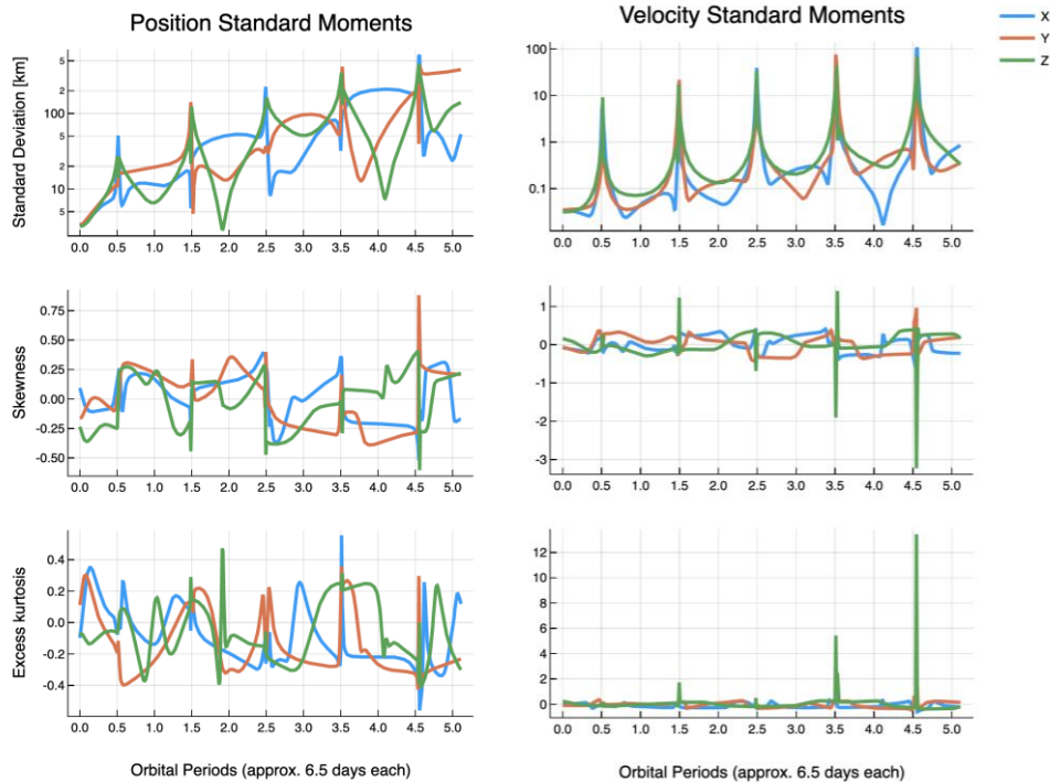
Figure 2. Evolution of position and velocity standard moments over time in an NRHO.
