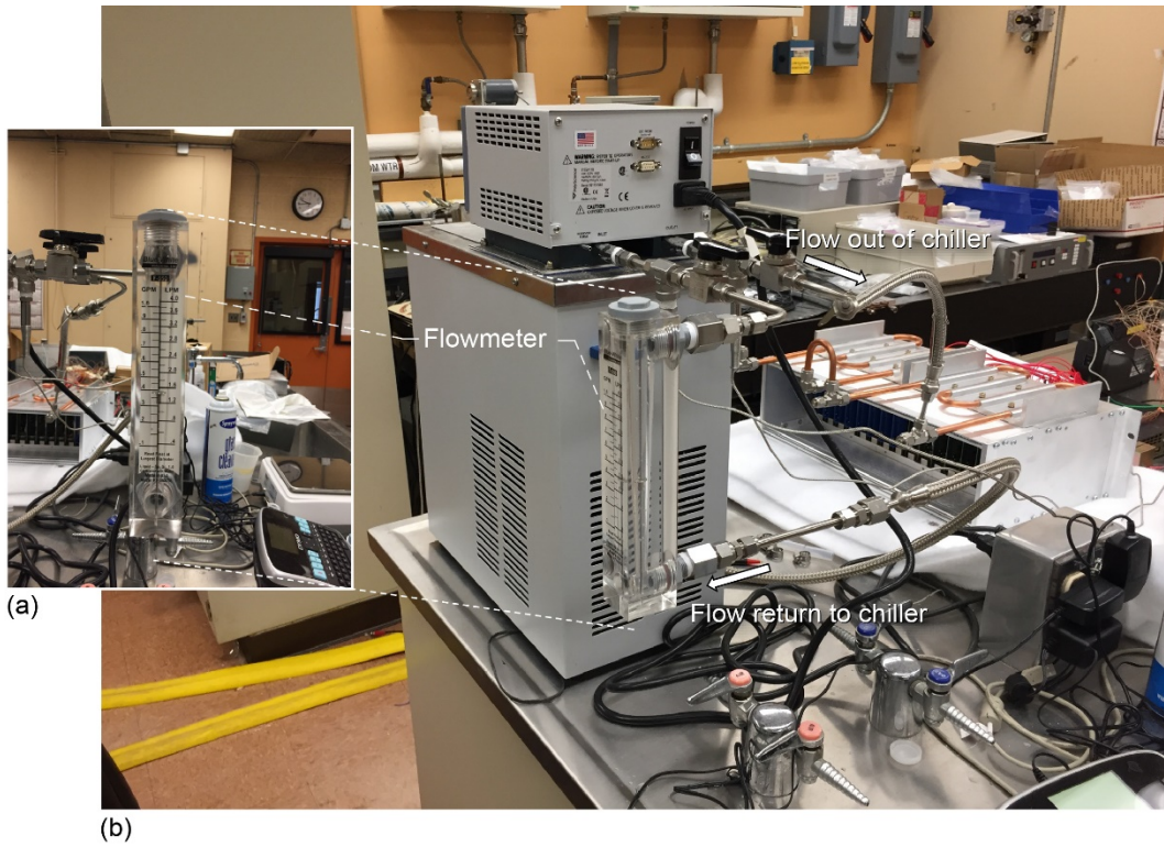
Figure 9.—Coolant system. (a) Flowmeter. (b) Recirculating bath.
