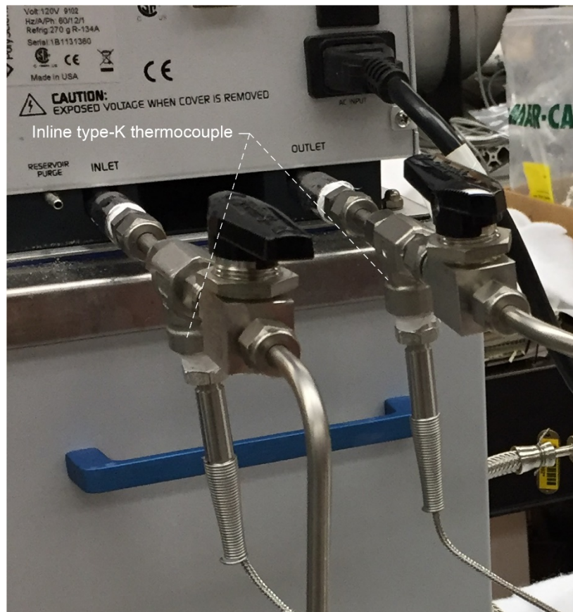
Figure 10.—Coolant inlet and outlet water temperature sensors.
