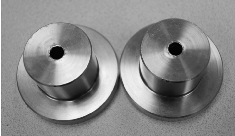
Figure 7. Steel pucks after all steel puck testing.
