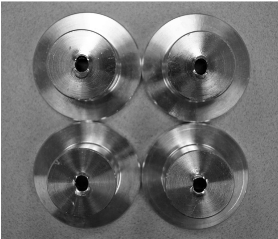
Figure 8. Representative aluminum pucks after use for two load cases (top: cases 111-1 and 111-2; bottom: cases 105-2 and 105-3).
