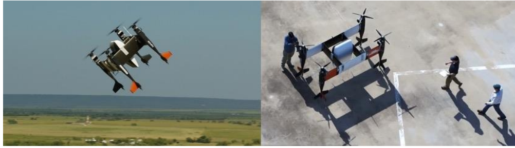
Figure 33. Bell's 70 lb. payload eVTOL autonomous pod transport, APT70. Images courtesy of Bell
