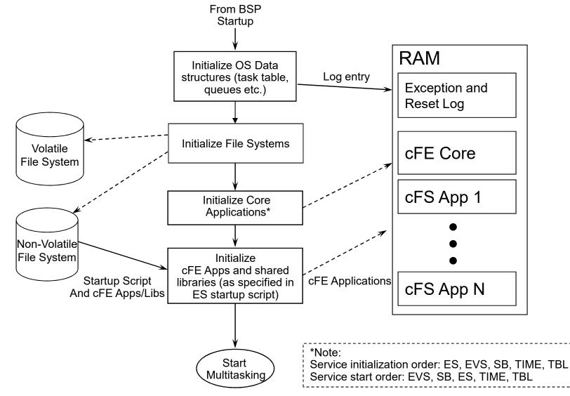
The cFE core is started as one unit. The cFE Core is linked with the RTOS and support libraries and loaded into system EEPROM as a static executable.
