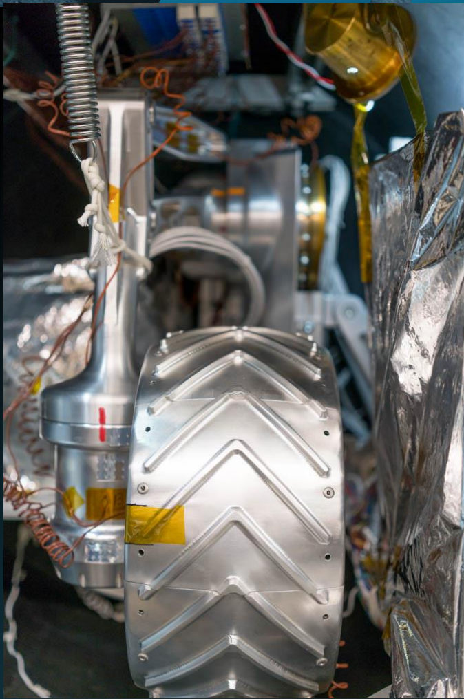
TVAC chamber testing of VIPER rover wheels & steering assemblies @ NASA-JSC
