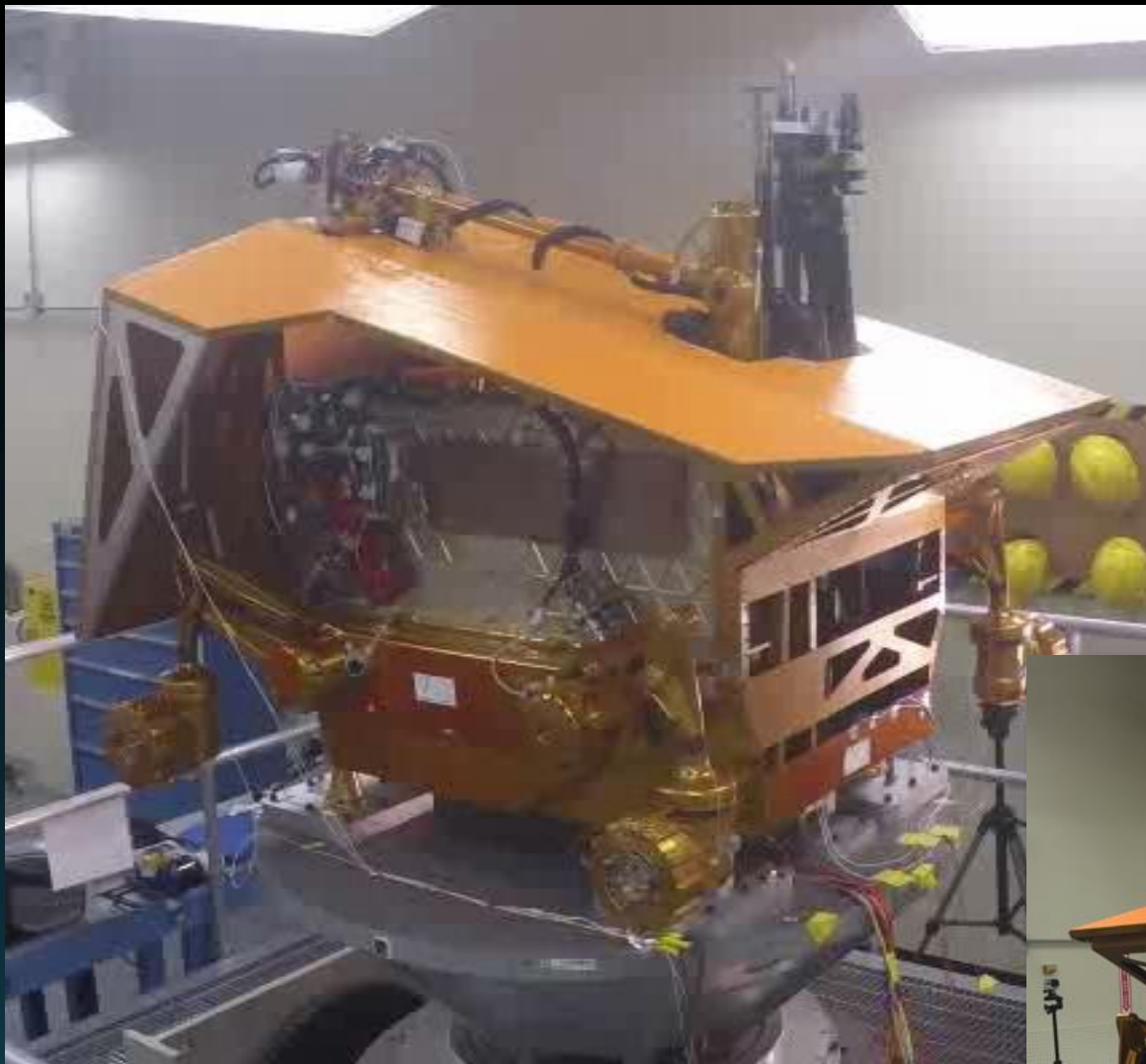
TVAC chamber Z-axis testing of VIPER rover
