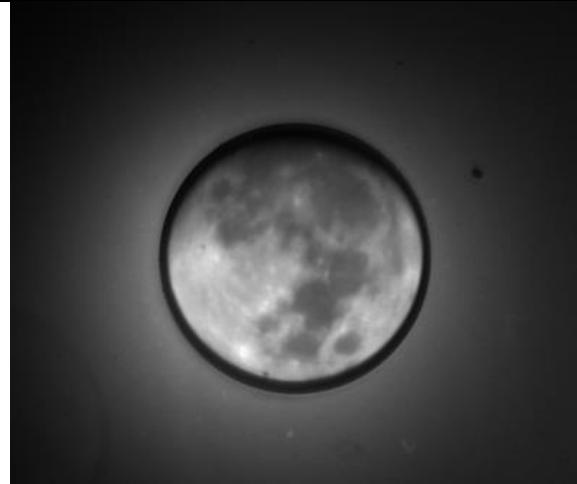
Figure 1. Example of an observation of the Na corona (with occulting disk in place) and the unocculted Moon superimposed on the occulting disk. This image is not calibrated. The full Moon observation is taken either just before or just after the occulted image, and they are subsequently superimposed to determine the distance from the lunar limb to the occulting disk.
