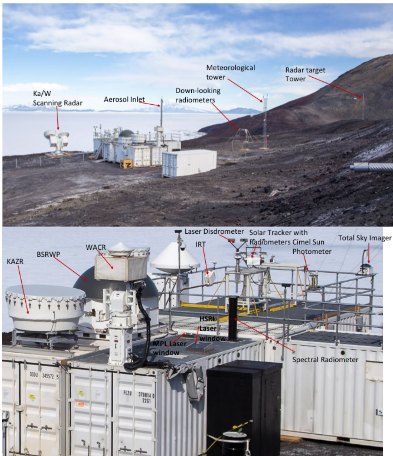
Figure 2. The AMF2 installation at the McMurdo Station CosRay site. Top: view of the entire site showing locations of adjacent meteorological and radar calibration target towers, and the southerly view of the scanning radars. Bottom: detail of instrument installation within the AMF2.
