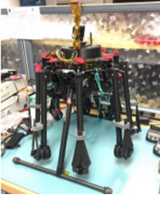
Fig. 6. DJI S1000 octocopter used for flight tests.
