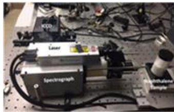
Fig. 2. SUCR Sensor with an ICCD camera, laser, spectrograph, collecting optics and a target sample.
