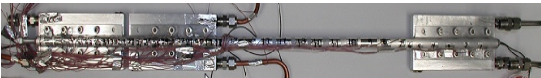
Figure 2.—Gas-charged heat pipes demonstrated freezing and thawing of aluminum and ammonia heat pipe condenser.
