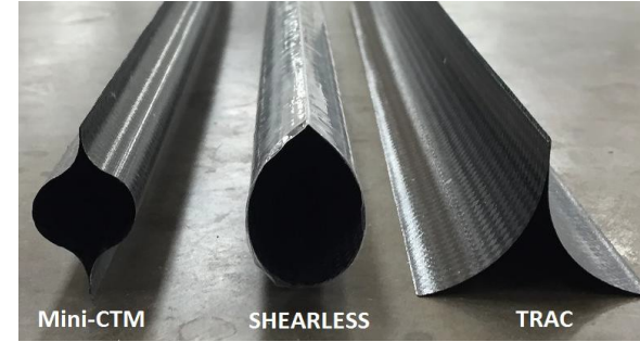
Rollable HSC booms under development at LaRC
