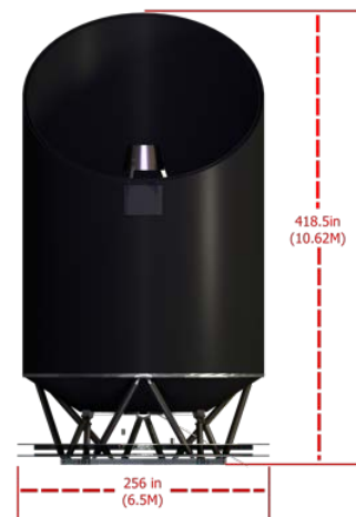
Figure 5. Origins CPM dimensions
