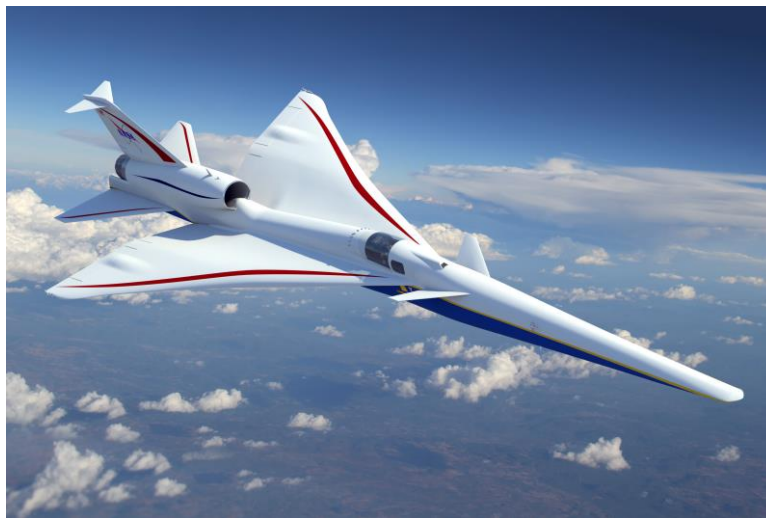
Figure 1. (Loubeau_QueSST.jpg) Artist rendering of a NASA design for a low-boom demonstrator aircraft, exhibiting a characteristic slender body and carefully shaped swept wings.
