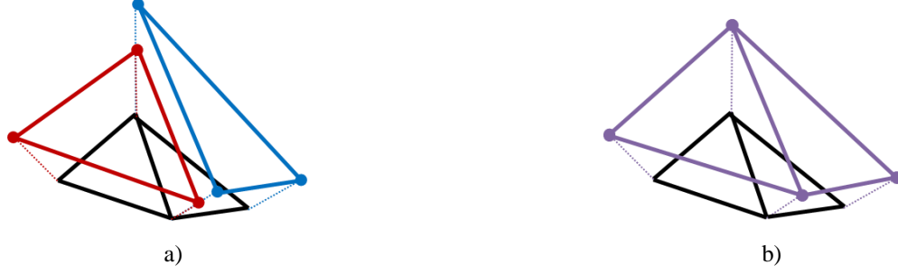
Figure 5: Depiction of the Surface Extrusions a) Before the Node Based Smoothing and b) After the Node Based Smoothing
