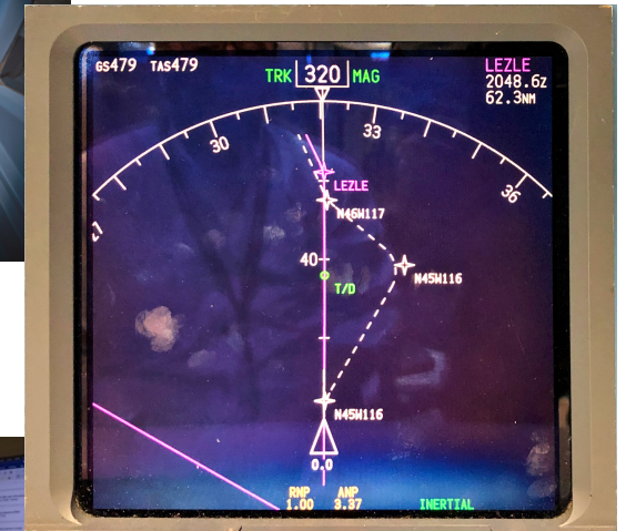
TAM route clearance on B777 Nav Display – Boeing IASL
