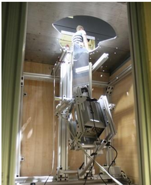
Fig. 3. Lower surface camera and mirror system with open viewport
