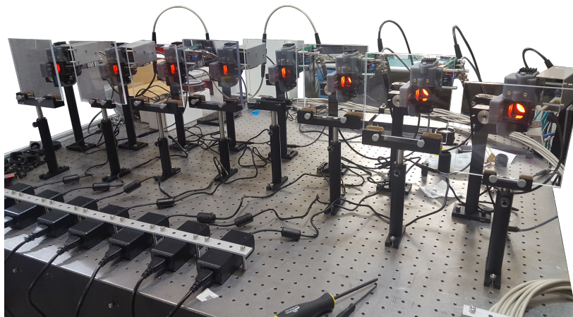
Fig. 4 All eight cameras triggering synchronously, each with an acrylic window that is used in the mock-up to simulate the ARC tunnel windows.
