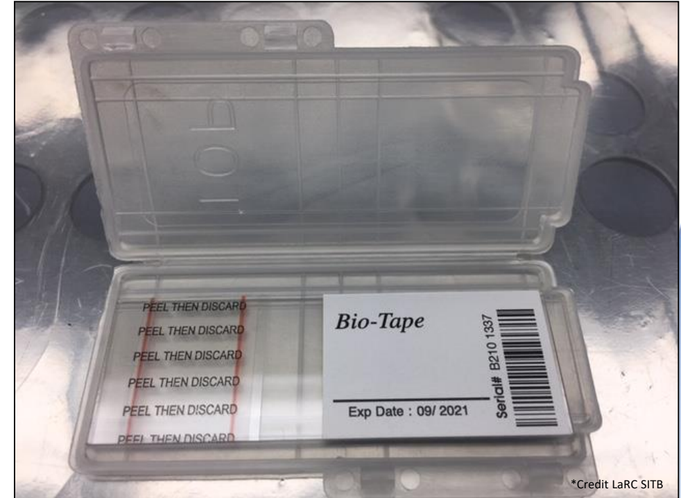
Unused commercial biological tape lift slide inside case
