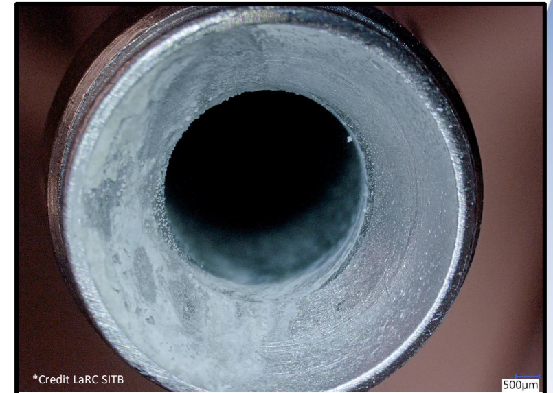
Contamination residuals on MEDLI2 Supersonic Tubing Assembly hardware
