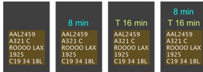
Fig. 1. TOBT and TMAAT Advisories were shown in the form of countdown timers on the new ATD-2 ramp controller decision support tool, the Ramp Traffic Console (RTC). From left to right they are 1) baseline, no advisories, aircraft information only, 2) gate advisory (TOBT) shown in cyan ("8 min"), 3) spot advisory (TMAAT) shown in green ("T 16 min"), and 4) both gate and spot (TOBT+TMAAT) advisories displayed.
