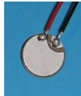
Example: UT sensor 7mm Diameter 0.2mm thick
