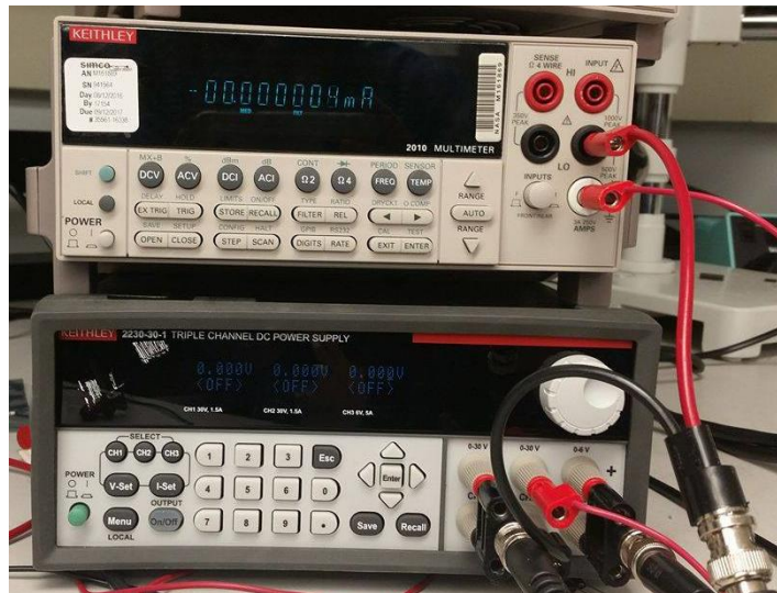
Figure 5. Keithley multimeter (top) and three channel power supply (bottom) used
