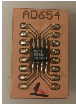
Figure 2: AD654 in an SOIC 8 package soldered to a daughter card for ease of testing.
