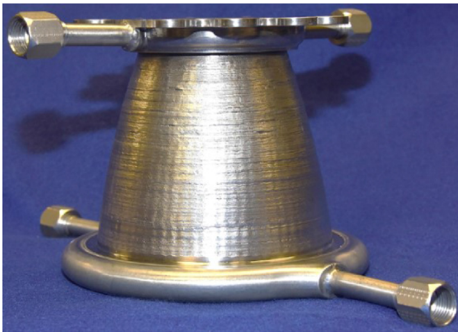
Fig. 4. LWDC closeout of monolithic, inco 625.
