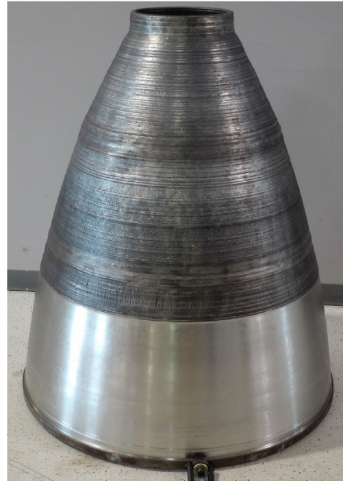
Fig. 18. 1/2-Scale RS-25 Nozzle Liner fabrication with Blown Powder DED (~44" dia and ~50" tall).
