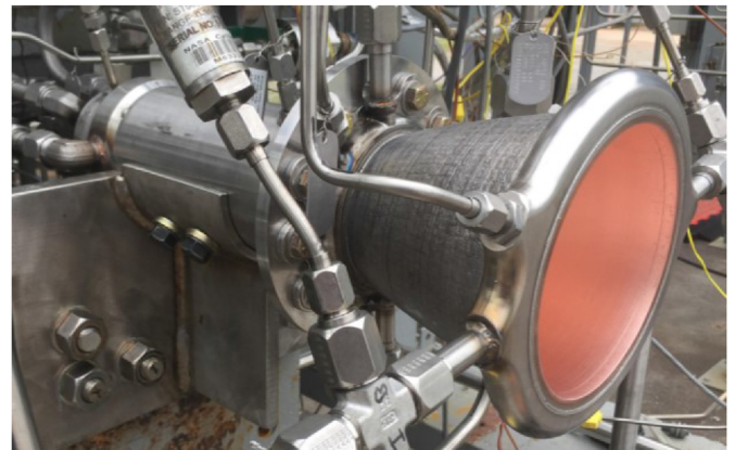
Fig. 13. Bimetallic LWDC nozzle at NASA Test Stand115.
