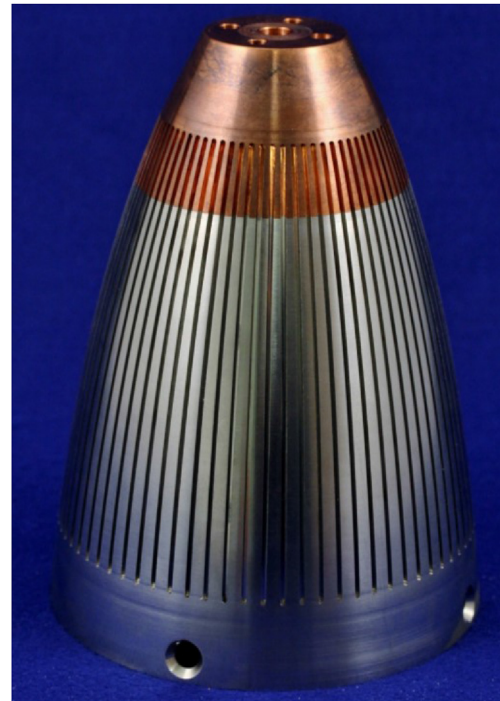
Fig. 11. Explosive bonded axial bimetallic liner.
