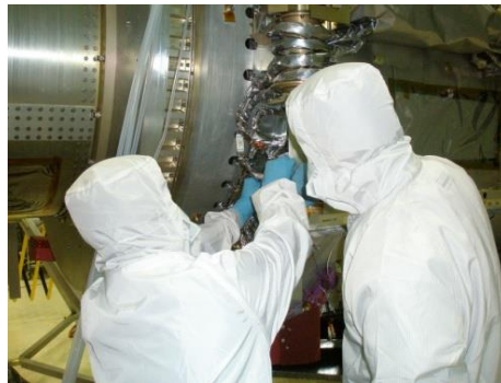
Installing Thermal Insulation on Spacecraft in Clean Room (space blankets)
