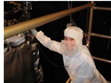
Assisting with Setting Up Test Equipment inside Thermal Vacuum Chamber, Preparation for 28- day thermal test
