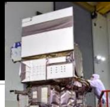
Radiators (white panels)
