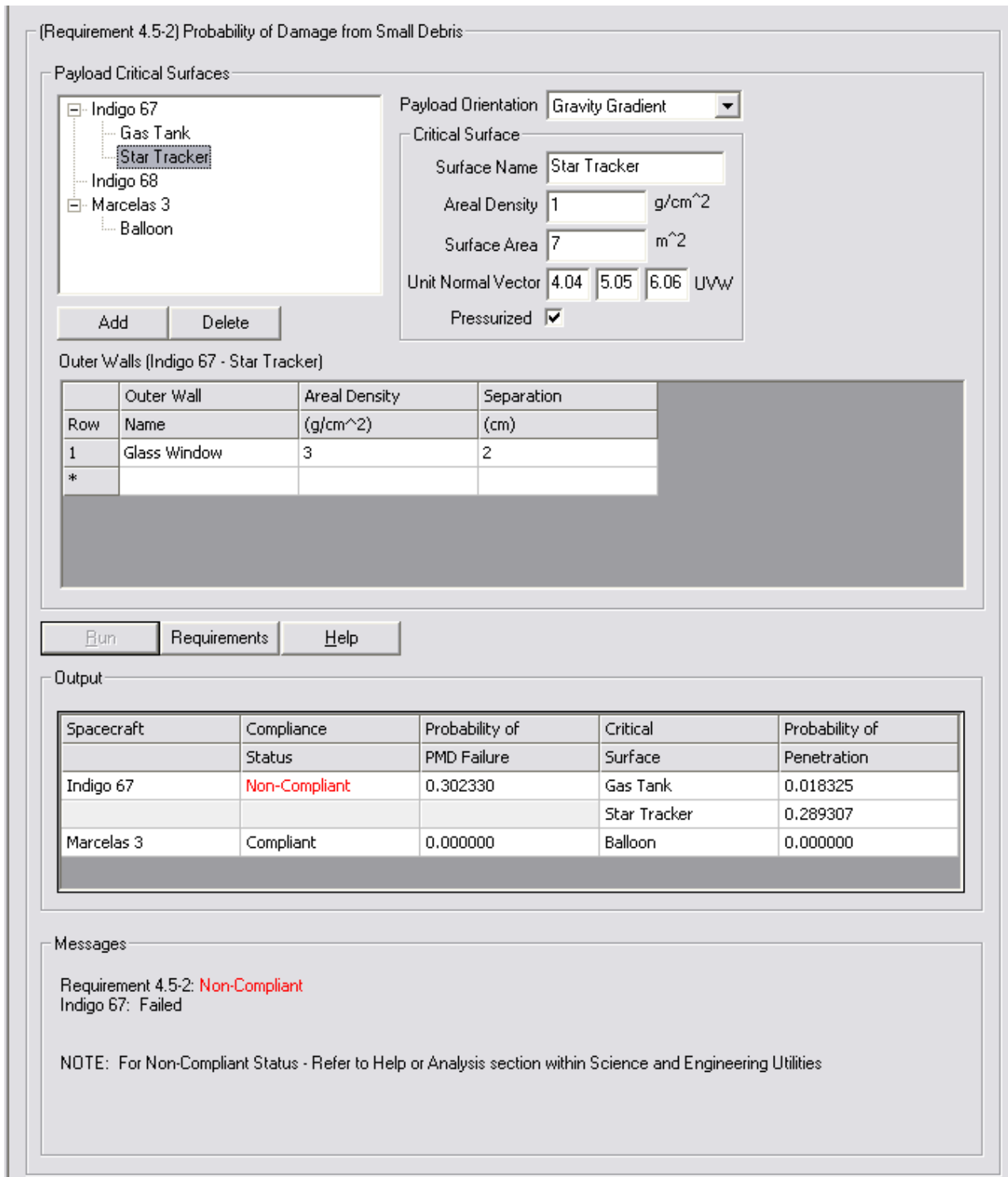
Figure 3 - 4: Requirement 4.5-2 Probability of Damage from Small Debris Dialog
