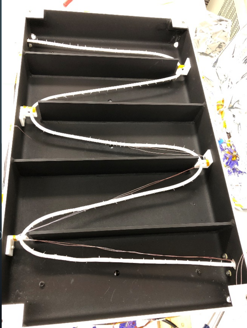
Temperature Controlled Shroud with Wire Bundle Test Article
