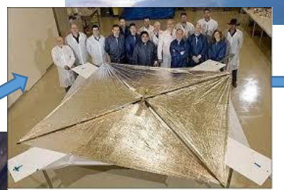
SMD In-Space Propulsion Technology Project 400 m 2 solar sail demonstrator Deployed at Plumbrook Station (2000 – 2003)
