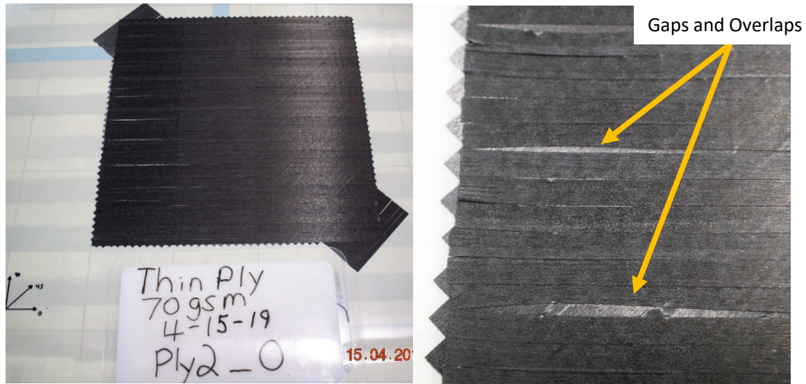
Figure 4. (a) Ply 2 with fiber angle 0^\circ . (b) Tow wandering in ply start.
