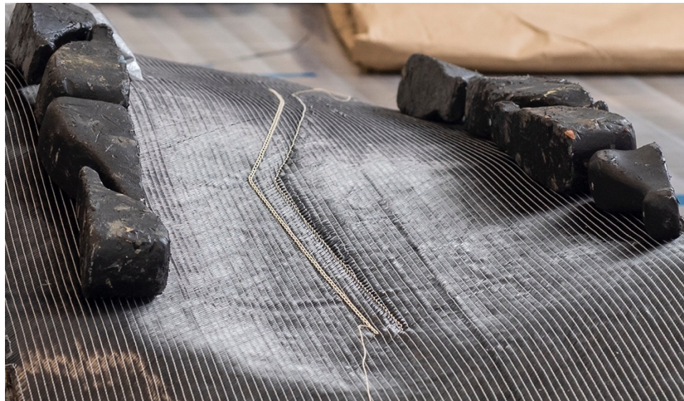
Figure 17. Two views of doubly-curved path demonstrator article representative of the NTF wind tunnel blade.
