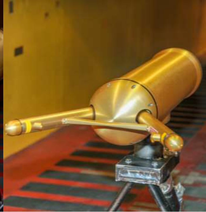
Optical Array Probe OAP-230Y 50 – 1525 \mu\text{m}
