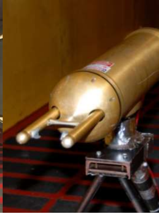
Optical Array Probe OAP-230X 15 – 450 \mu\text{m}
