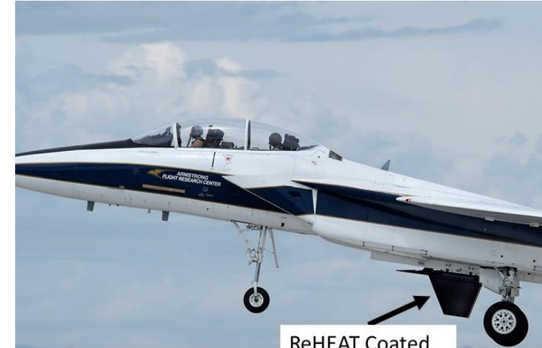
ReHEAT Coated Test Article
