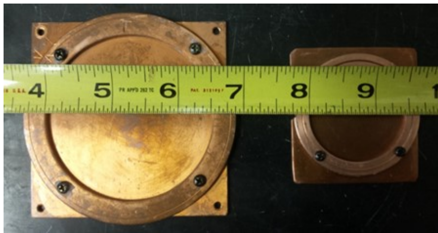
Fig. 10: Copper sample molds: 2.5 in. and 1.375 in. diameters.
