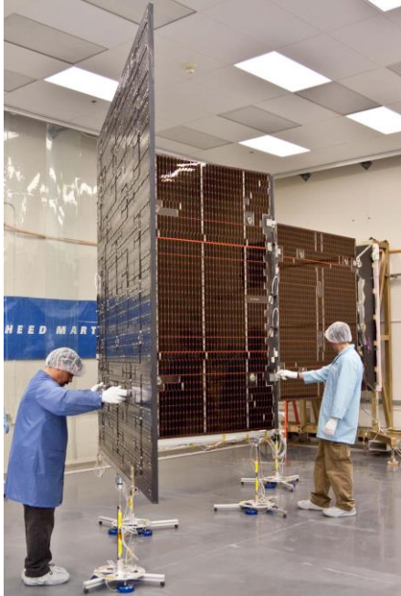
Figure 1: Typical rigid panel solar array as shown for the Juno spacecraft (Credit: NASA)
