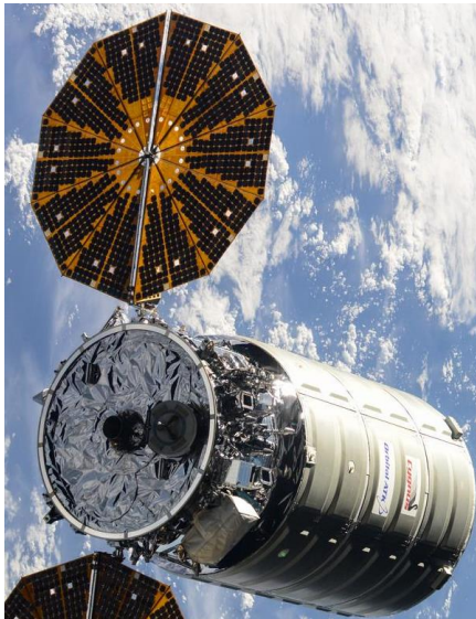
Figure 2: Ultraflex solar array in Earth orbit on an ISS Cygnus cargo module (Credit: NASA)
