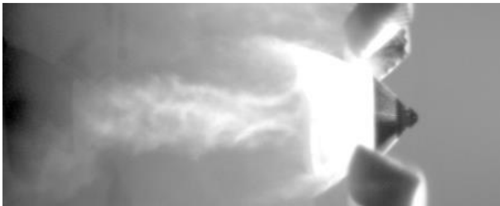
Figure 19: High-speed video frame capture of sabot separation in shot 2815 (axisymmetric steel drag skirt).
