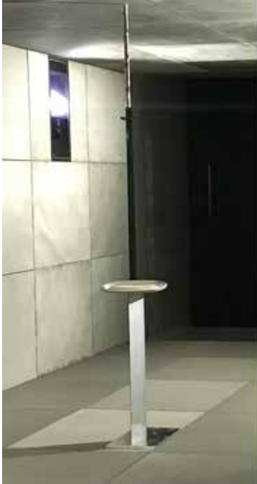
Fig 4. Array and sound source Set up in GRC 9-by15-Ft Aero-Acoustic Wind Tunnel.
