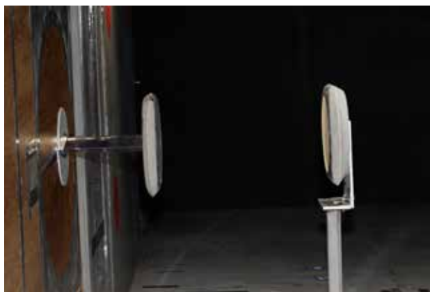
Fig 2. Array and source set-up in test section of Army 7-by10-Ft Wind Tunnel at ARC.
