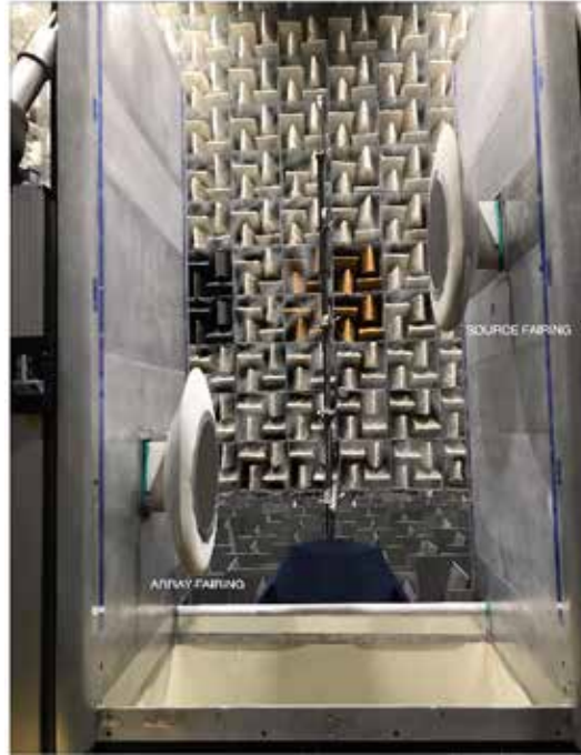
Fig. 5. Array and source fairings mounted on sidewalls of the LaRC Quiet Flow Facility nozzle.
