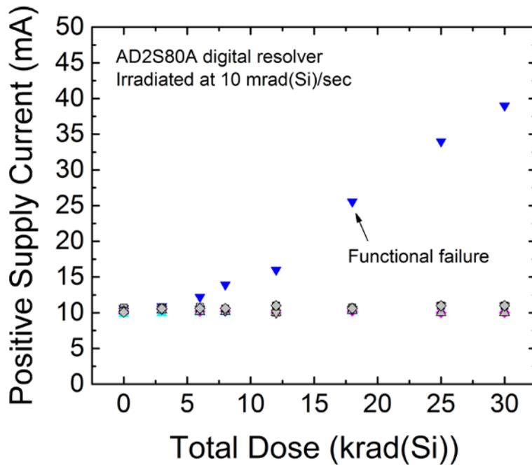
Figure 6. Positive supply current vs. total dose for devices irradiated at 0.01 rad(Si)/sec. Color symbols and gray symbols represent parts irradiated with bias and without bias, respectively. Functional failure occurred for one part irradiated under bias after 18 krad(Si). All other devices remained functional up to 30 krad(Si).
