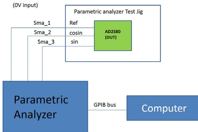
Figure 4. Block diagram of the measurement test setup.
