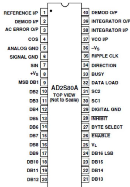
Figure 1. Pin configuration.
