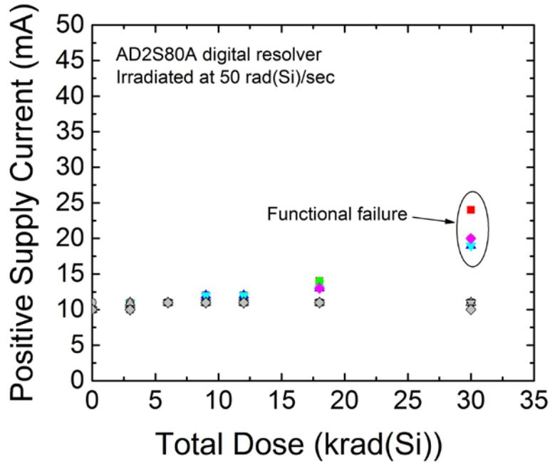
Figure 5. Positive supply current vs. total dose for devices irradiated at 50 rad(Si)/sec. Color symbols and gray symbols represent parts irradiated with bias and without bias, respectively. Functional failures occurred for all parts irradiated under bias after 30 krad(Si).
