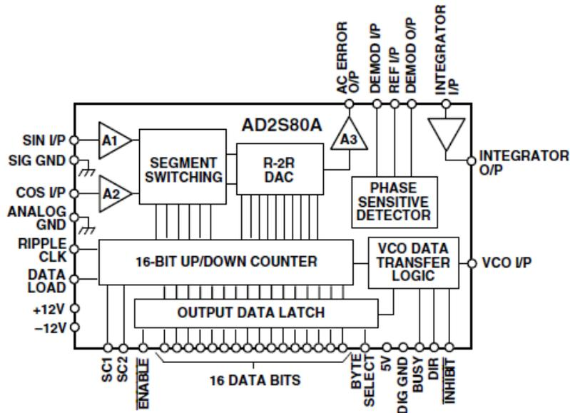
Figure 2. Functional diagram.
