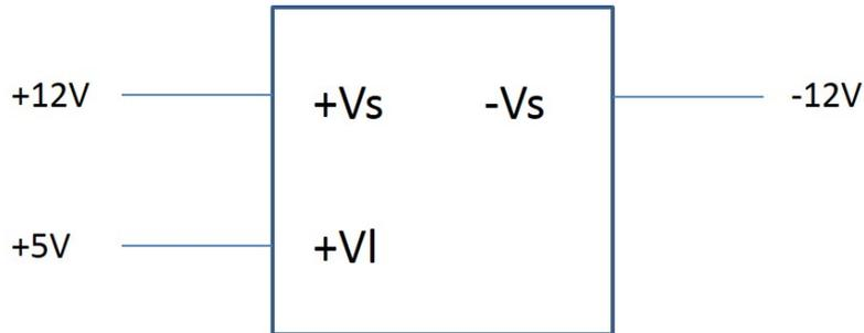
Figure 3. Schematic diagram of the irradiation bias configuration.
