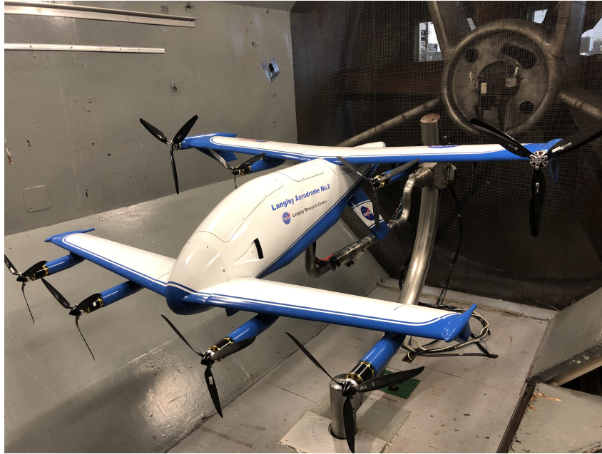
Figure 1. LA-8 UAS in the 12-foot low-speed tunnel.
