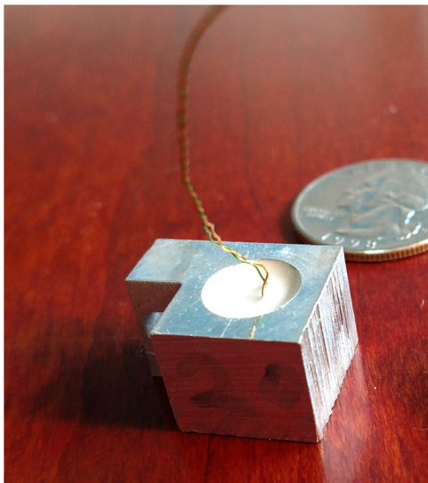
Fig. 2 A control thermometer for the NEID TMC. A 2N2222 transistor, operated as a diode, is potted in a small aluminum block with thermal epoxy.
